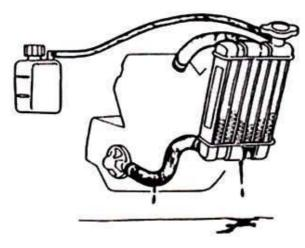
Coolant recommended: SYM Bramax radiator agent Concentration: 50% Radiator capacity: Main radiator: 850 c.c. Reserved tank: 420 c.c.
