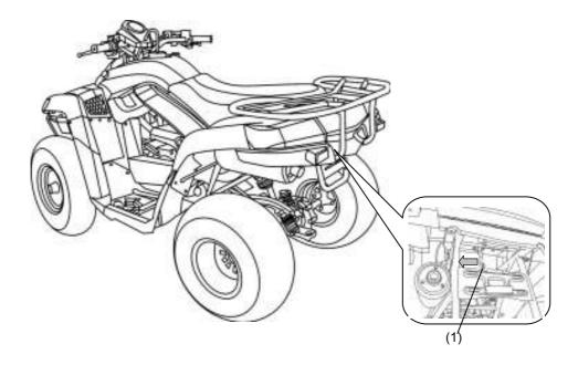
Pull the seat lock lever(1) at the Underneath of the seat.
