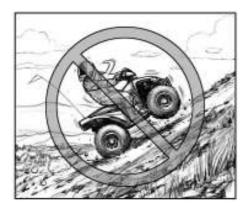
If your ATV has stalled or stopped and you believe you can continue up the hill, restart carefully to make sure you do not lift the front wheels which could cause you to lose control. If you are unable to continue up the hill, dismount the ATV on the uphill side. Physically turn the ATV around and then descend the hill.
