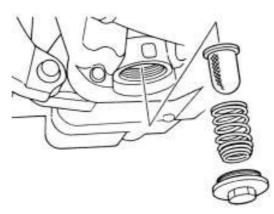
Open the filter nut assembly of the element, and remove the element. Remove the foreign materials from the element by using a gasoline or air spraying gun.
