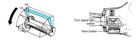
(4). Do you rotate the throttle valve handle while (5). Turn the ignition switch key "ON", and press horn pressing starting the button? button down, if the horn does not sound, the fuse may have been blown.
