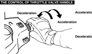
Acceleration : To increase speed. When riding on an inclined road, turn the throttle valve handle slowly to allow the engine to output its power.
