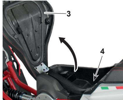
**NOTE:** After opening the compartment under the saddle, the key can be removed from the lock.
